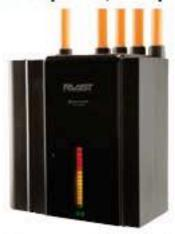
The FAAST XT 9400X can support a network of up to four pipes to protect as much as 28,800 square feet per detector, making it ideal for large open spaces, such as warehouses, atriums and cold storage units. Its pipes can run a total length of nearly 1,100 feet, with a maximum of 400 feet per single pipe. Long pipe runs enable the FAAST XT 9400X to be placed in a much more easily-accessed area for maintenance and testing, as opposed to common spot detectors. *Notifier*.
